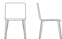
Poltrona monoscocca, base 4 gambe legno Mono-shell chair, 4 oak wood legs L 50/43 P 50/40 HT 81 HS 46
