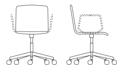
Poltrona monoscocca, base Loop 5 razze Mono-shell chair, 5 races Loop base L 68/47 P 68/43 HT 80/90 HS 44/54
